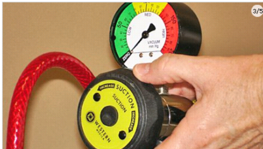
Turn the wall suction dial to adjust the amount of suction.
